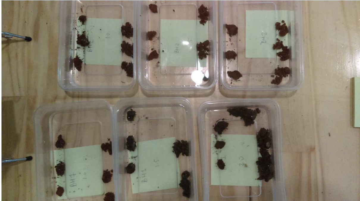
Soil slaking after 24 hours in distilled water.
